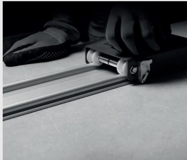
CUTTING DETAIL WITH GUIDE ON SLAB
